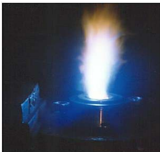
Adapted from [30] Figure 14. Plasma torch producing high temperature plasma
